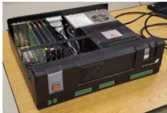
**Figure 2.** Robotic arm controller
